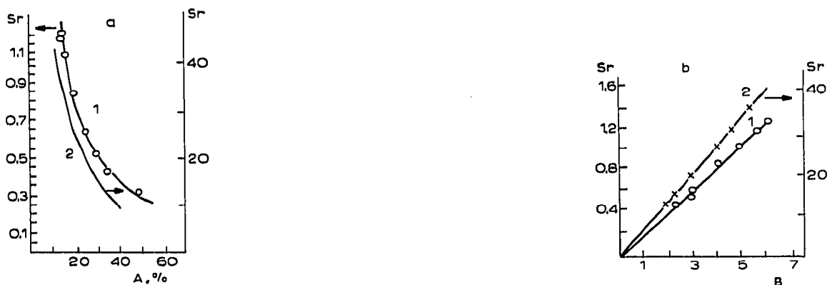
Fig. 7. (a) Calibration graph from ref. 7 for copolymers of vinyl acetate with butyl maleinate (1) and copolymers of vinyl acetate with butyl acrylate (2). (b) Calibration graph plotted from the data in graph (a) by re-calculation with the aid of eqn. 1. A, content of butyl ether; B, ratio of components in copolymer (vinyl acetate/butyl maleinate and vinyl acetate/butyl acrylate).
